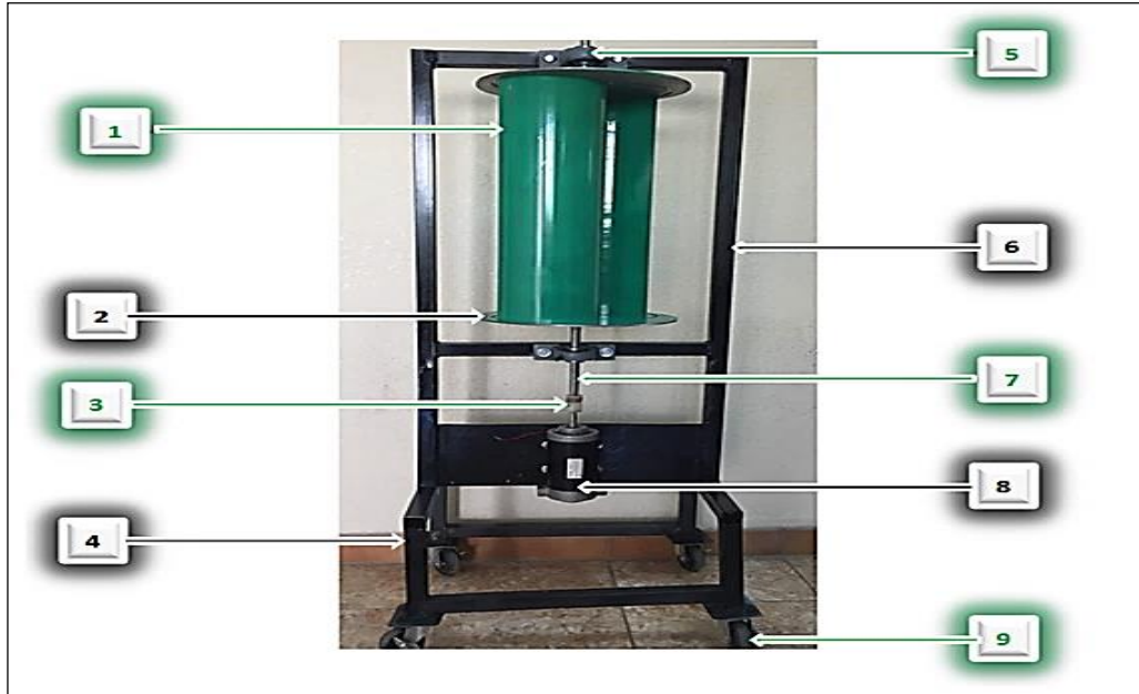
Figure 3. The design model of Savonius wind turbine with its accessories; (1) Turbine blades, (2) End plate, (3) Sleeves, (4) Base, (5) Bearing, (6) Frame, (7) Shaft, (8) Generator, (9) Wheels
