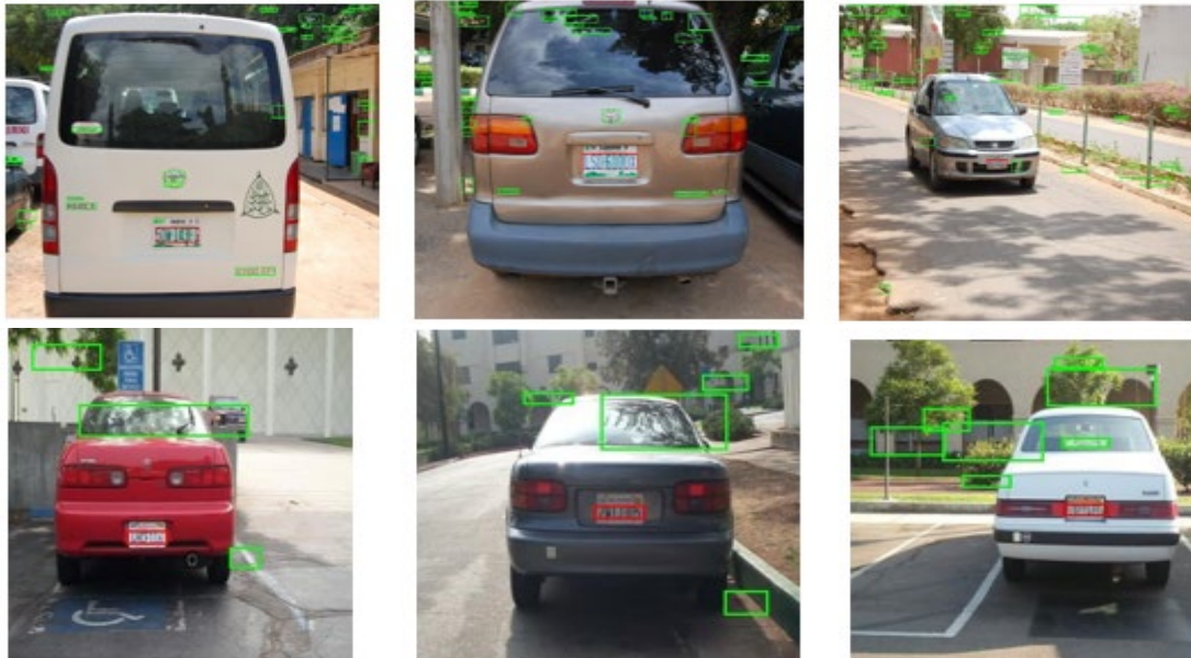
Figure 5. Vehicle images showing the localized plate number as indicated by the red bounding box, while the green is the other candidate regions.
