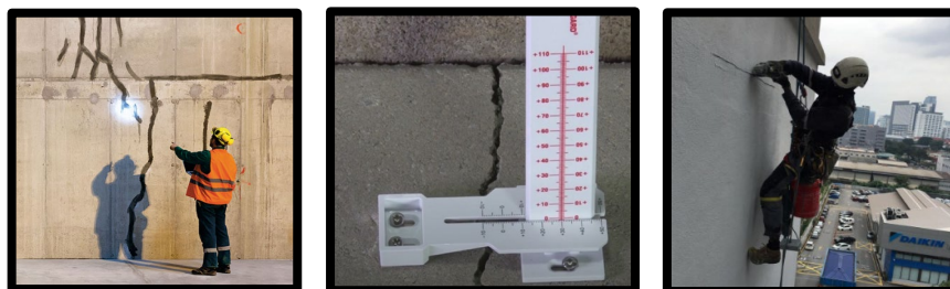
Figure 1. The current method for Structural Health Monitoring.
