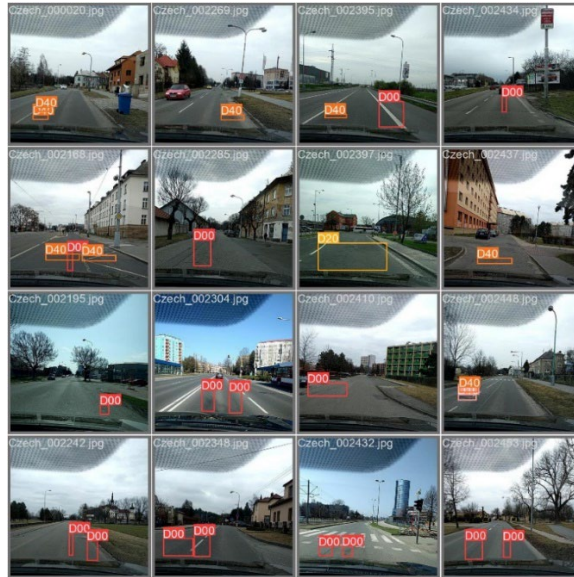
Figure 5. Road damage detection using SSA YOLOv8n.
