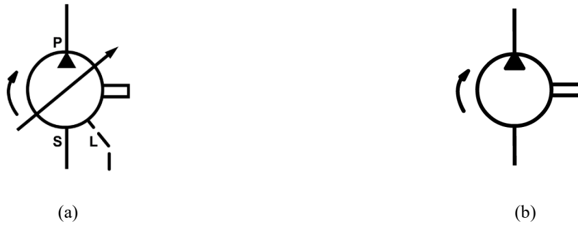
Figure 2. Schematic symbol for a hydraulic pump: (a) Variable displacement pump, (b) Fixed displacement pump.
