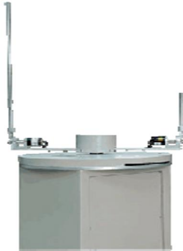
Figure 1. RDIP physical system (www.googoltech.com)
