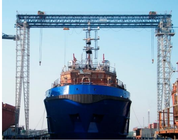
Figure 2. Gantry crane system
