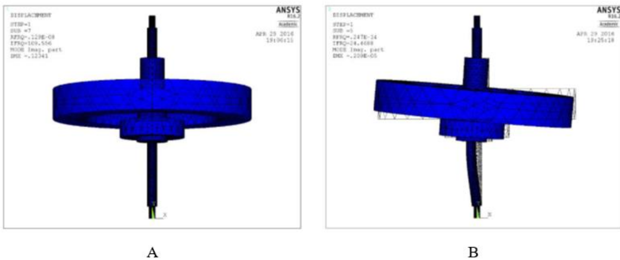
Figure 12. (A) Mode shape at critical speed N1 (685 rad/s, 109.56 Hz & FW stable) and (B) Mode shape at critical speed N2 (148 rad/s, 24.47 Hz & FW stable)
